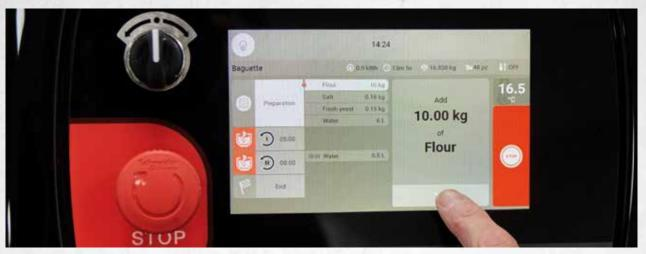
The Recipe mode provides **step-by-step instructions** for the mixing process. The user can program resting times and set reminders to add ingredients.
